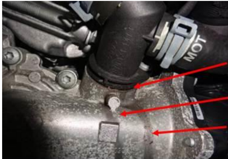
Figure 6. Areas where coolant marks can be found.
