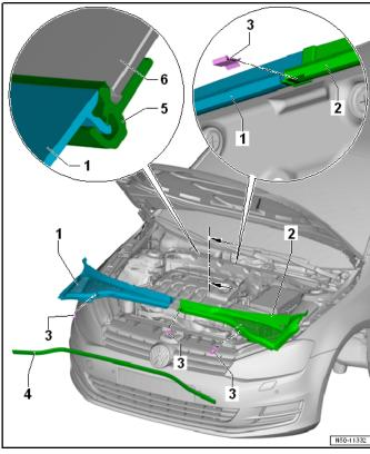
Reinstall plenum chamber cover in the reverse order of removal according to the ELSA Repair Manual.
