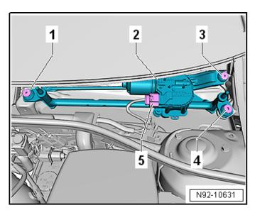
Reinstall wiper linkage in the reverse order of removal according to the ELSA Repair Manual.
