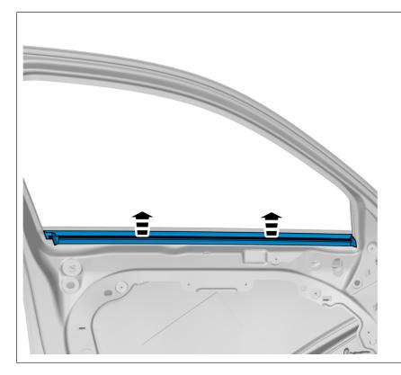
Remove the marked part. The part is not to be reused.
