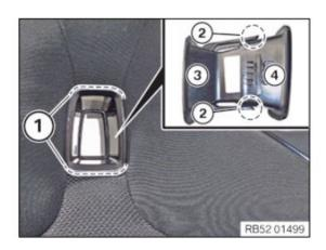
. Correctly position trim for the hatch (3) and (4) in the marked area (1).
