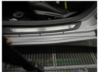
1. Starting at the rear of the door opening as shown, begin measuring towards the front of the vehicle.
