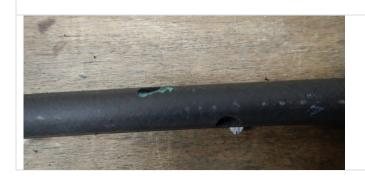
6. From the rearmost hole made in step 4, measure 20 mm **forwards** and mark the seal on the side which faces **down** when installed in the vehicle.
