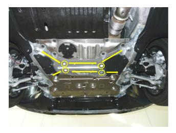
Blow out the front axle support at the openings (circled) with compressed air.
