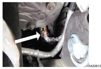
8. Plug the engine coolant heater cord assembly into the heater and secure it with the metal clip. Be certain the metal retaining clip is secured onto to the deeper of the two grooves.
