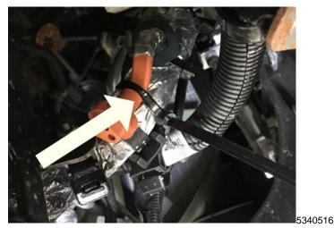
From underneath the vehicle, locate the engine coolant heater power cord. It is on the front passenger side of the engine block. Cut the wire tie securing the engine block heater power cable. Remove and discard the wire tie. (shown without the shrink tube installed).
