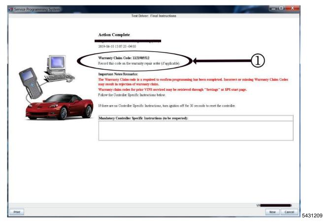
**Important:** To avoid warranty transaction rejections, you MUST record the warranty claim code provided on the SPS Warranty Claim Code (WCC) screen on the job card. Refer to callout 1 above for the location of the WCC on the SPS screen.
