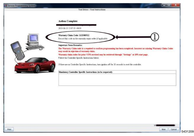
**Important:** To avoid warranty transaction rejections, you MUST record the warranty claim code provided on the SPS Warranty Claim Code (WCC) screen on the job card. Refer to callout 1 above for the location of the WCC on the SPS screen.
