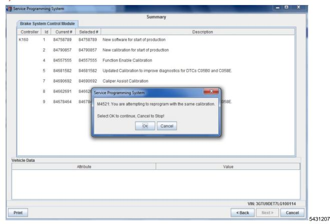
**Important:** If the Same Calibration/Software Warning is noted on the SPS screen, select OK and follow screen instructions. After a successful programming event, the WCC is located in the Service Programming System dialogue box of the SPS Summary screen. No further action is required. Refer to the Warranty section of the bulletin.
