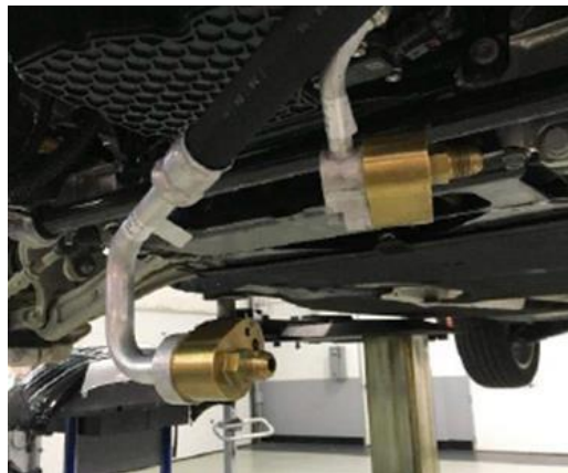
Figure 6. Installation of VAS 6338/3 and 6338/12.
