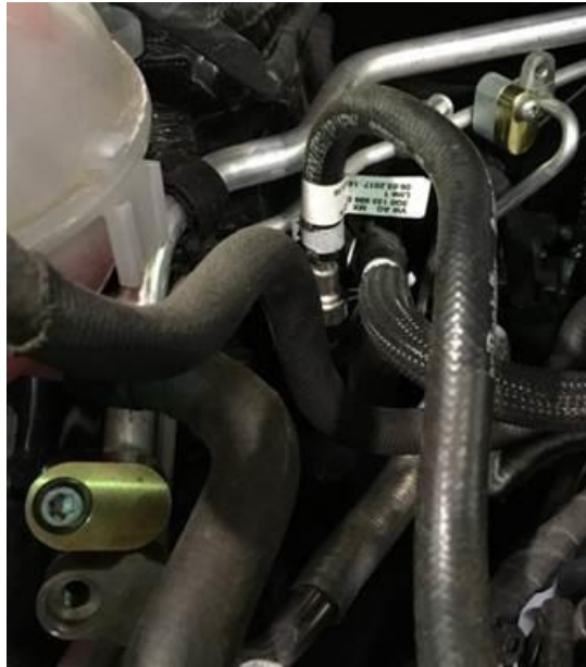
Figure 4b. Installation of Low side rear A/C Line connection block adaptor VAS 6338/5
