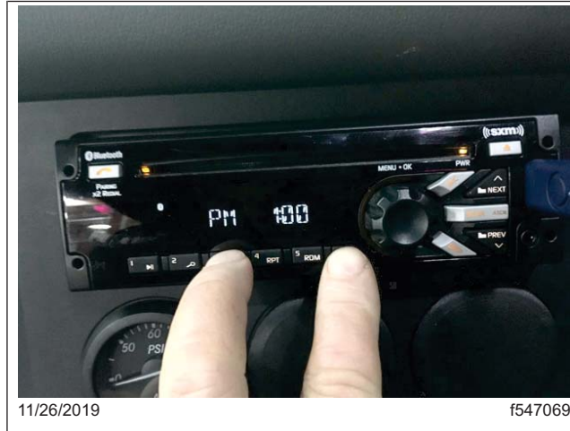
Fig. 2, Holding Buttons 3 and 6
