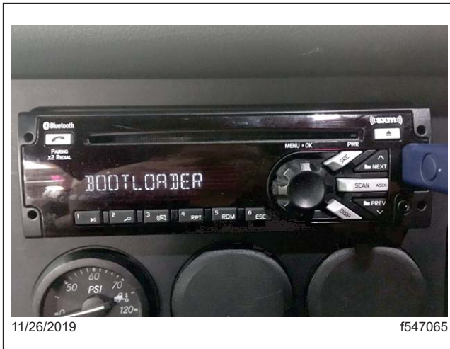
Fig. 3, Radio Displaying "Bootloader"
