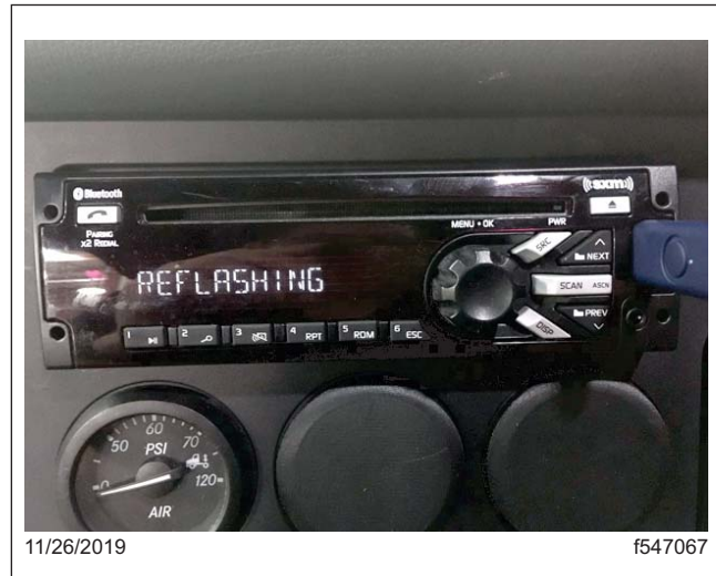
Fig. 4, Radio Displaying "Flashing"
