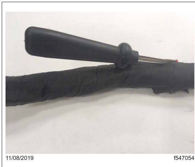
Fig. 9, Cutting an Opening into the Fiber Wrap
