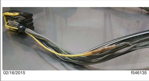
Fig. 5, Splicing the Wires
