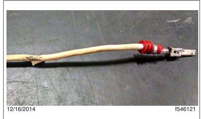
Fig. 2, Insulation Discoloration, Major
