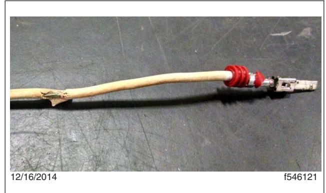
Fig. 2, Insulation Discoloration, Major
