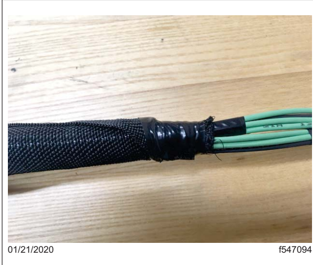
Fig. 7, Harness Wrapped with TwistTube®
