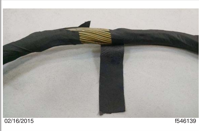
Fig. 11, Unwrapping the Harness
