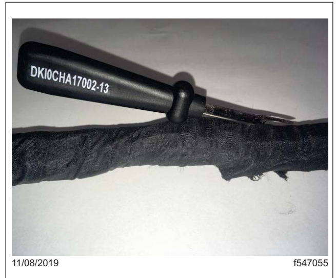
Fig. 10, Cutting the Fiber Using the Blunt End of the Seam Cutter
