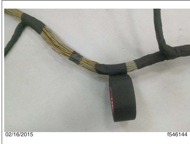
Fig. 14, Wrapping the Harness with Fiber Tape
