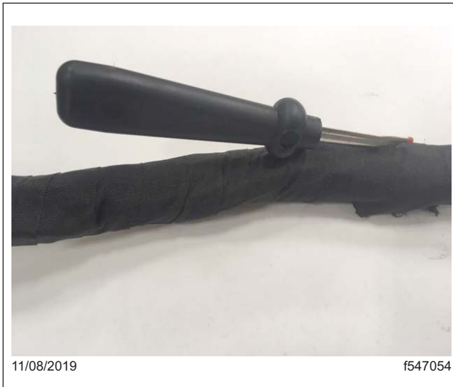
Fig. 9, Cutting an Opening into the Fiber Wrap
