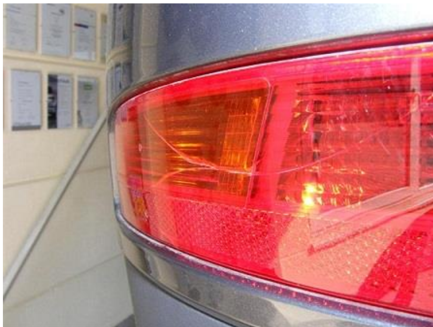
Figure 5. Turn signal in rear bumper cracked.
