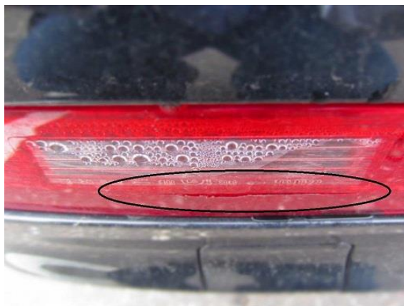
Figure 3. Turn signal in rear bumper cracked.
