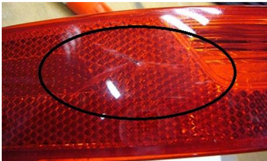
Figure 4. Turn signal in rear bumper scratched or cracked.
