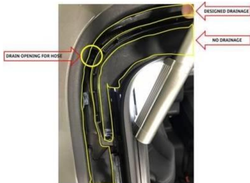
Figure 7. Sunroof water channeling diagram.
