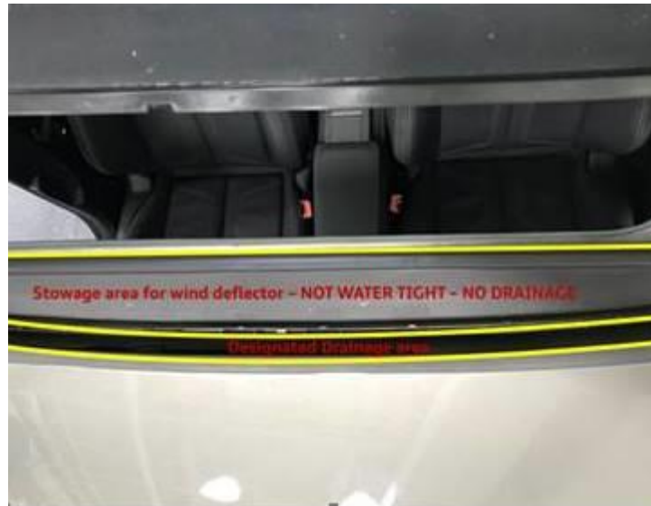
Figure 6. Areas of sunroof opening water elimination capabilities.
