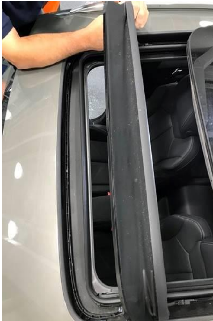
Figure 5. Front sunroof opening with drainage exposed.
