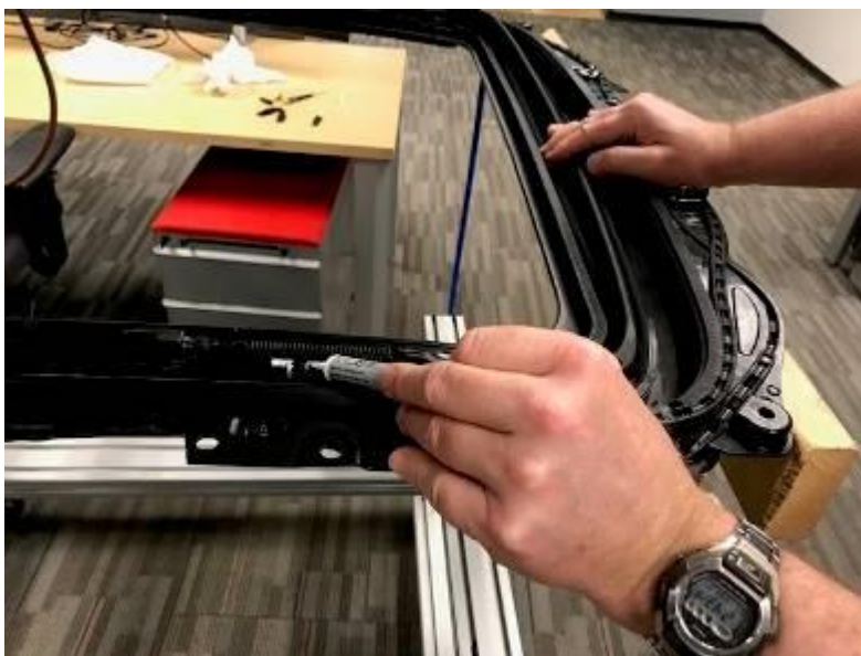
Figure 10. Lubrication points, wind deflector compressed.
