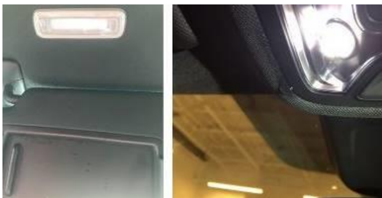
Figure 1. Water intrusion near the headliner.
