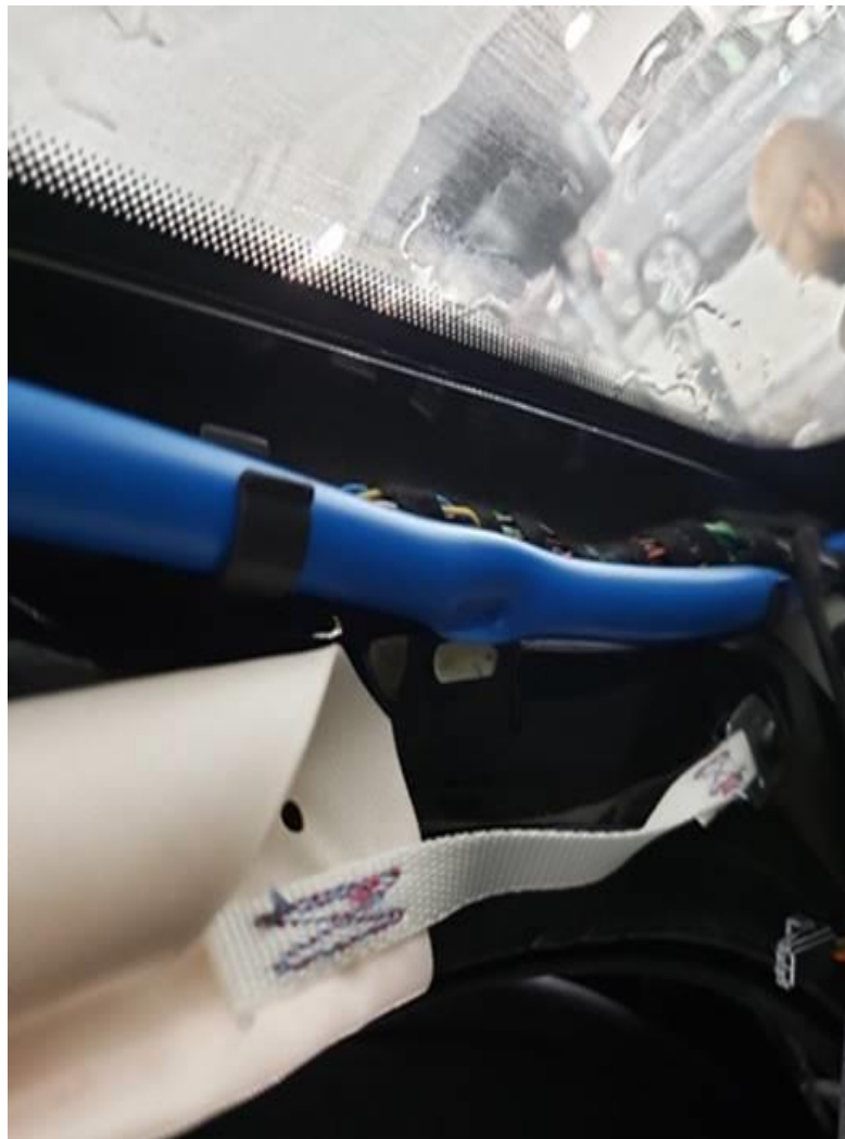
Figure 2. Sunroof drain hose pinched by pillar trim.
