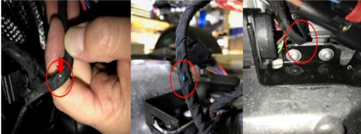
Figure 2. Body harness inspection near the area of transmission connector.
