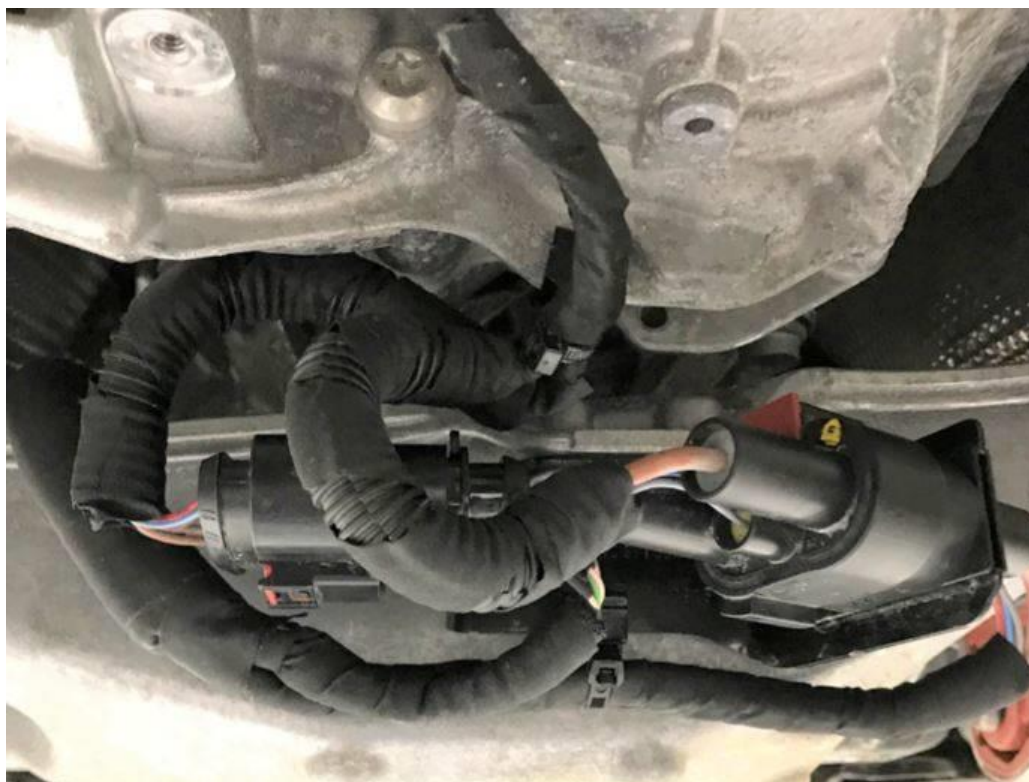
Figure 17. Fully wrapped corrugated tub and final harness routing.
