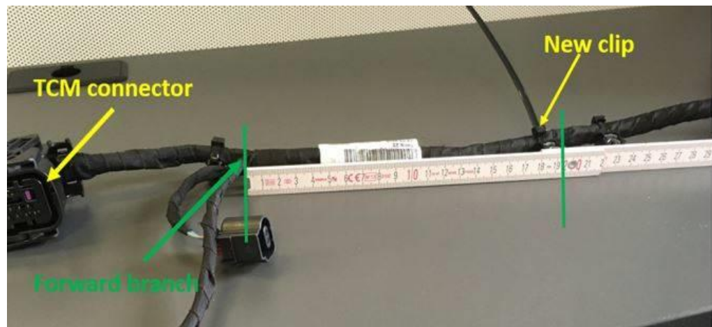
Figure 5. New clip fitted 195mm from the forward branch of the transmission harness.
