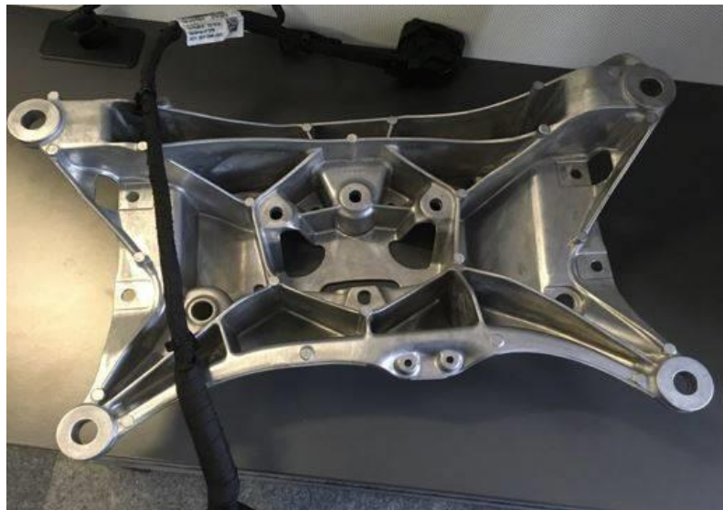
Figure 11. New harness routing and clip locations.
