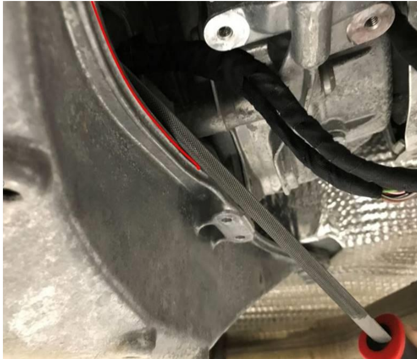
Figure 10. Deburring of the transmission cross brace.
