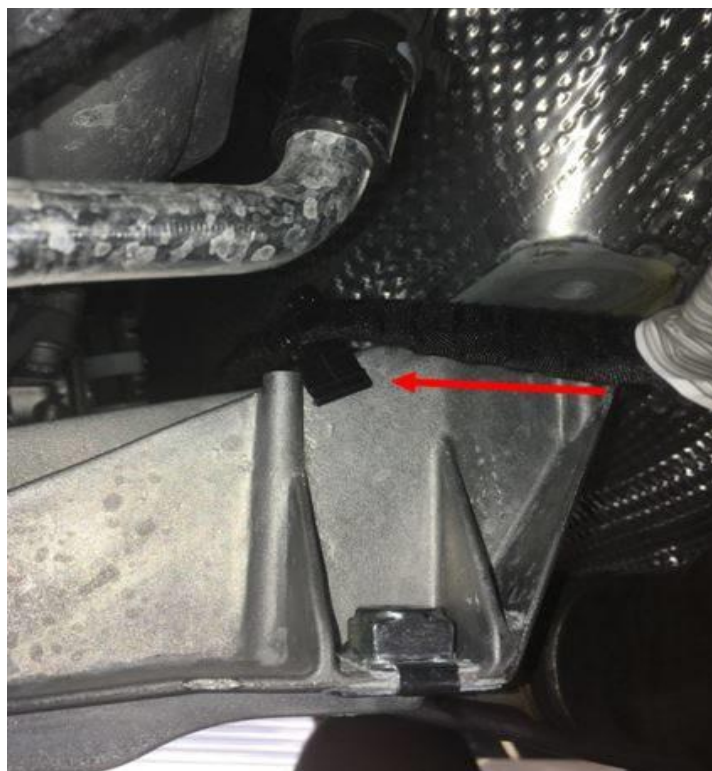
Figure 12. Attachment point of forward clip.
