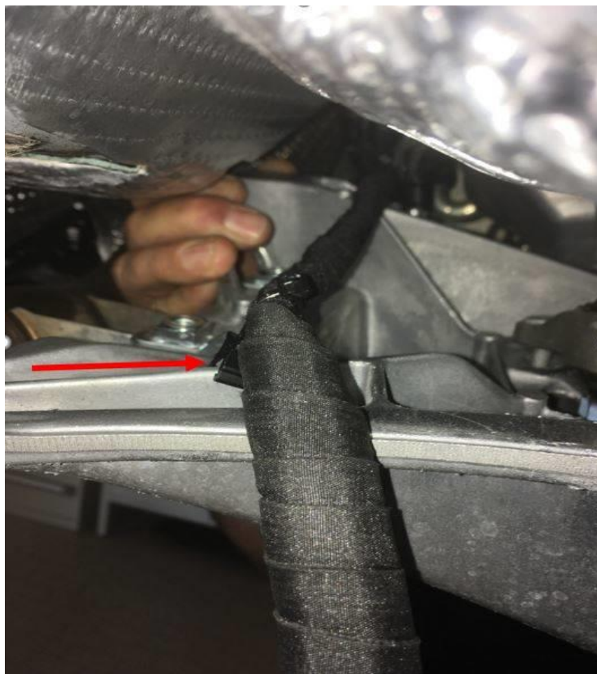
Figure 13. New routing and clip location.
