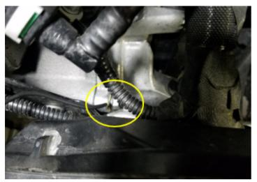
6. When procedure is complete the ground wire should look lik e the installed wire below:
