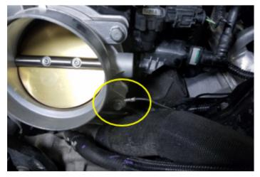
5. Attach the other end of the ground wire to the rock er cover fastener as shown in picture below with the crimp side of the ring terminal facing towards the bolt head:
