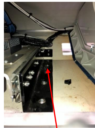
Screws securing tray in place in the rear
