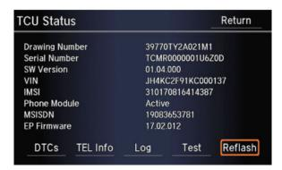
12. On the TCU Reflash screen, select Software Update and wait for the system to enter the reflash mode.
