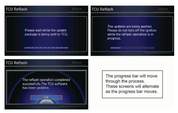
14. Once the reflash is complete, select **OK** and remove the USB flash drive.
