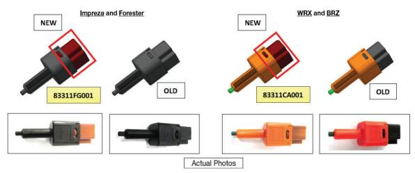
The new switches can be identified by a brownish -colored harness connection socket as opposed to black.
