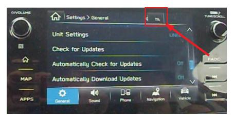
1.6.1) Wait until the download progress reaches 100%. During the software download, the H/U is fully functional. **NOTE:** It is normal for the progress to hang at some points for 1-2 minutes. This does not indicate a concern. **BE PATIENT**.
