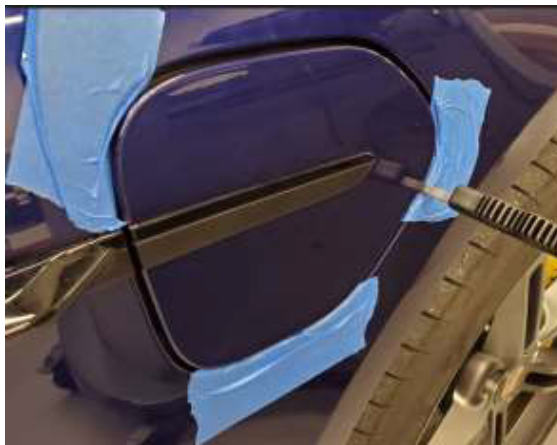
Disengaging the front retaining clip
