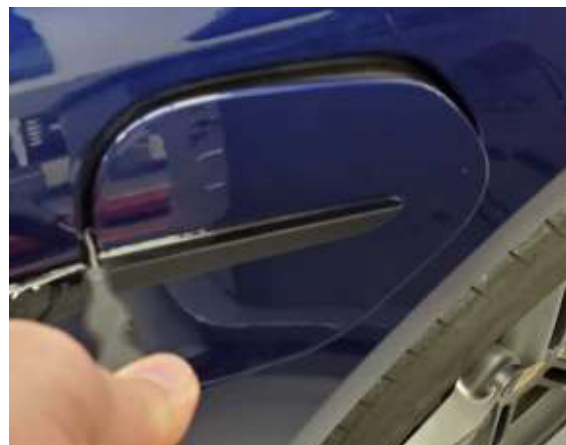
Disengaging the upper rear clip
