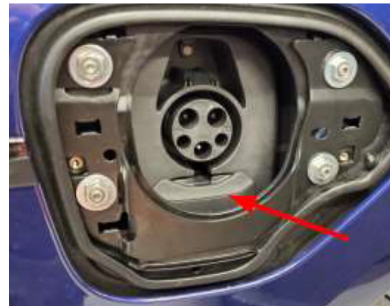
View with charge port door removed. Note that the flap for DC charging terminals is still blocked by the door frame. Only AC charging is possible
