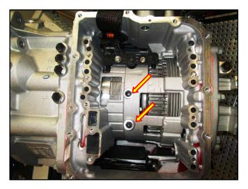
19. Align the manual shaft to the shift lever and install the valve body.
