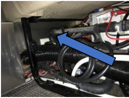
Run the wire through the back of the dinette seat.
