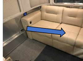
The wire will run under the lounge to the 12VDC power panel.
