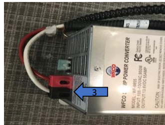
Two wires will need to be removed from the power center. The first, wire-1(6 gauge) in the picture above, runs to the 12VDC power panel under the lounge. The second, wire-2(8 gauge), runs to the converter. A third white wire, wire-3 (8 gauge), will need to be removed from the converter. Cap off all three wires, as they will not be used. Run a new 6-gauge ground wire connected directly to the converter, torqued to 25-35 inch-pounds, and run straight to the 12VDC power panel.
