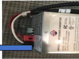
To run the second wire, you will need to access the converter by removing the panel below the wardrobe and then remove the power center.
