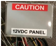
The 12 volt power panel under the lounge has the main grounding bar for the 12 volt system.
