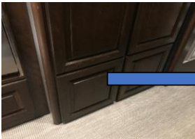
To run the second wire, you will need to access the converter by removing the panel below the wardrobe and then remove the power center.
