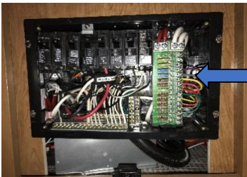
Two wires will need to be removed from the power center. The first, wire-1(6 gauge) in the picture above, runs to the 12VDC power panel under the lounge. The second, wire-2(8 gauge), runs to the converter. A third white wire, wire-3 (8 gauge), will need to be removed from the converter. Cap off all three wires, as they will not be used. Run a new 6-gauge ground wire connected directly to the converter, torqued to 25-35 inch-pounds, and run straight to the 12VDC power panel.
