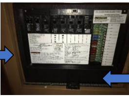
To run the second wire, you will need to access the converter by removing the panel below the wardrobe and then remove the power center.
