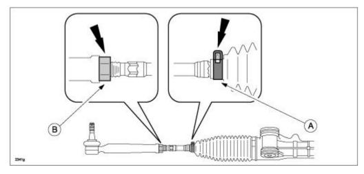
10. Rotate the tie-rod to adjust the steering wheel center. Refer to the following charts for rotating direction.
