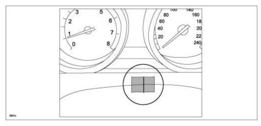
6. Drive the vehicle and align the steering wheel to its driving center, then put another mark on the tape.
