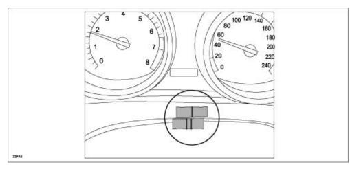
7. Measure the distance between the two lines. The offset can be approximately calculated using 1mm = 1° of offset.
