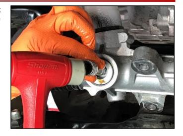
16. Reinstall the yoke spring (J) removed in step 10 of this procedure.
