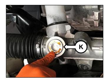
15. If necessary, use a short socket extension and a rubber mallet to seat the yoke assembly (K) fully.
