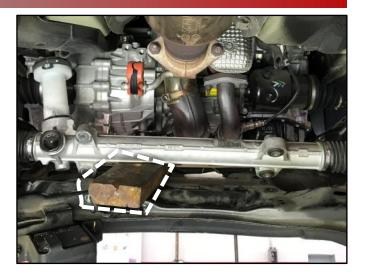
8. Remove the locking nut (H) using the locking nut removal tool (57718 2W009FFF).
