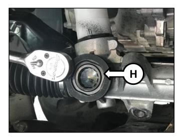
Using the 24mm hexagon bit socket (HXD24), remove and discard the yoke plug (I) and discard.
