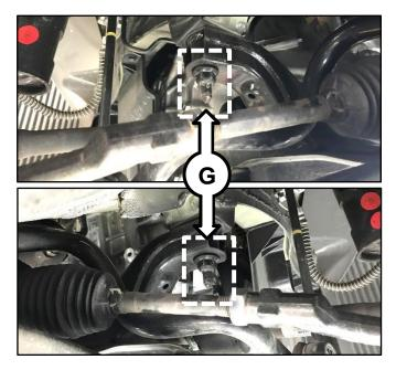
6. Remove the four (4) stabilizer bar mounting bolts at the subframe.
