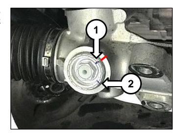
20. Loosen the plug approximately 1/4 of an inch and align the mark on the housing with groove 2 (blue mark #2) of the plug.
