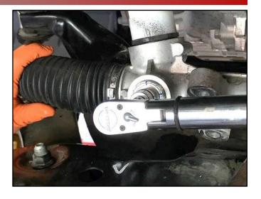
19. With a marker, mark a line on the housing in line with groove 1 (blue mark #1) of the plug.
