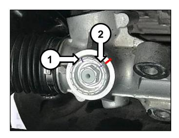
21. Partially install the new locking nut (M) by hand to prevent cross-threading of the nut and plug threads.
