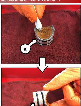
14. Install the improved yoke assembly (K) into the yoke housing and then apply a small amount of lubricant to the top of the yoke assembly.
