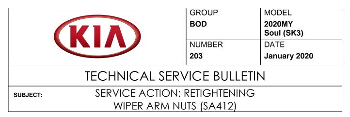
This bulletin provides the procedure to retighten the wiper arm nuts to the torque specification on some 2020MY Soul (SK3) vehicles produced from November 4, 2019 through December 12, 2019, which may not have been properly torqued during assembly. Before conducting the procedure, verify the vehicle is included in the list of affected VINs.
