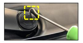
3. Tighten the <u>two</u> (2) left and right wiper arm retaining bolts (B) to specifications.
