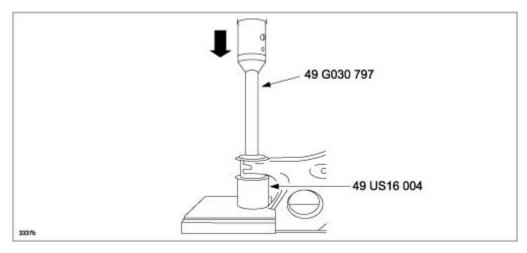
3. Install the new modified front lower arm bushing using SSTs.
