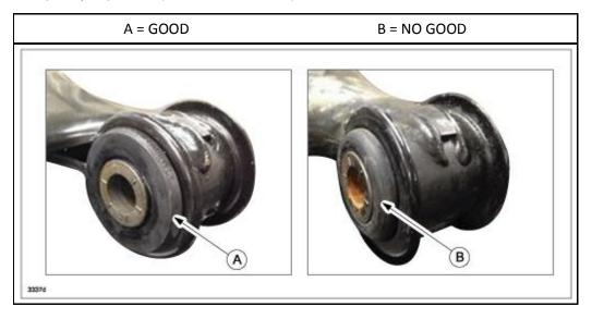
4. Verify that the new bushing is installed in the correct position by measuring the protruded part (A - B) as shown below.
