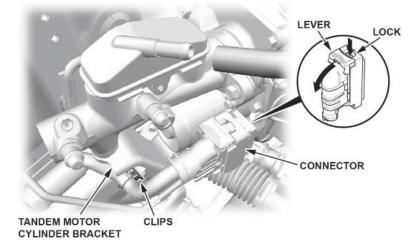
10. Remove the bottom bolt and side nuts from the tandem motor cylinder, and slide the rubber mount forward out of the tandem motor cylinder bracket. Remove the tandem motor cylinder without the bracket.
