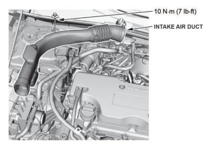
6. Remove the intake air duct bracket.
