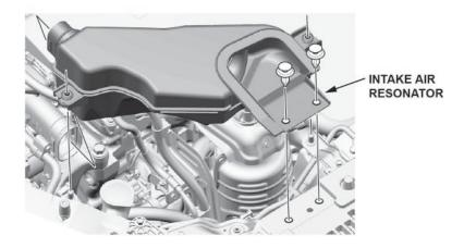
5. Remove the intake air duct.
