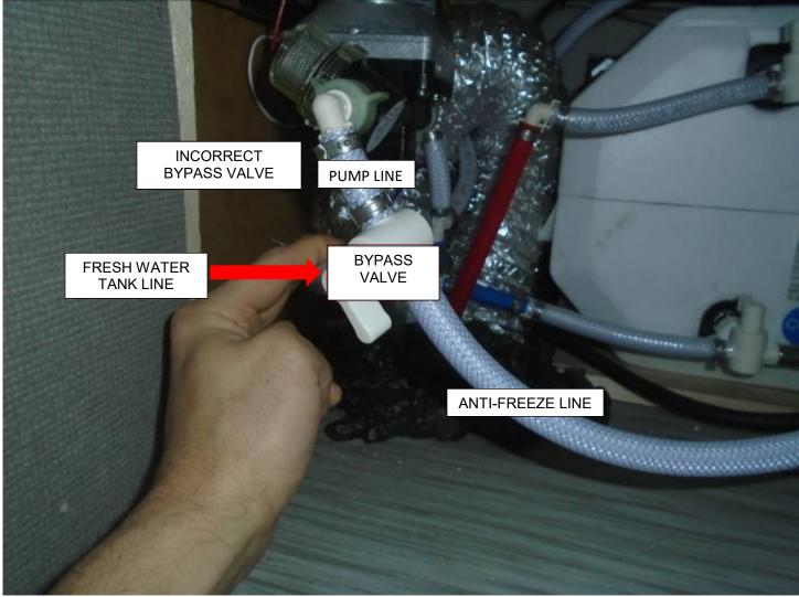
FOR CORRECT ORIENTATION OF THE BYPASS VALVE INSTALLATION, SEE THE NEXT PHOTO.
