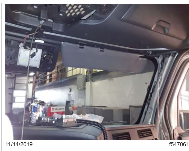
Fig. 1, Installing the OH Harness
