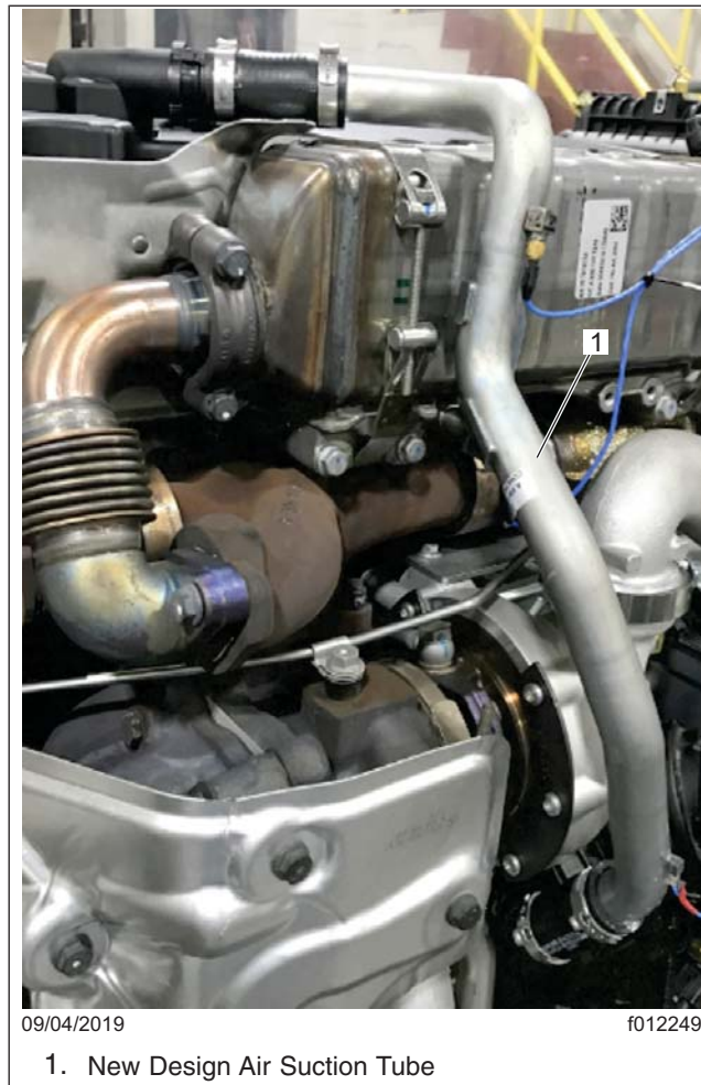
Fig. 2, Installing New Design Air Suction Tube
