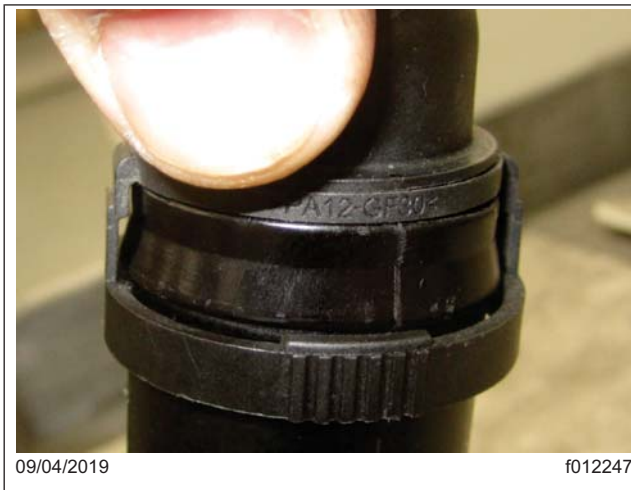
Fig. 1, Removal of the Air Section Tube
