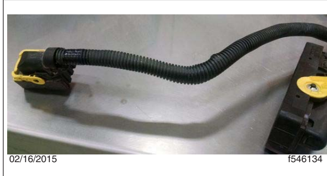
Fig. 7, Harness Wrapped with Convolute
