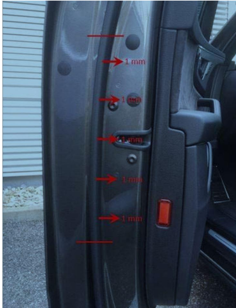
Figure 3. Install the new outer door seal with an inward offset by 1.0 mm.
