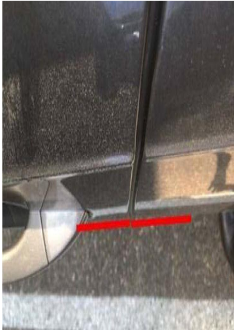
Figure 2. The front door can be flush or slightly underflush to the rear door.
