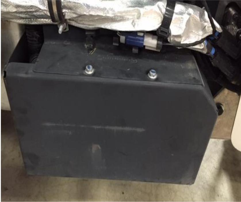
**Figure 14 – ACM Cover Installation**
