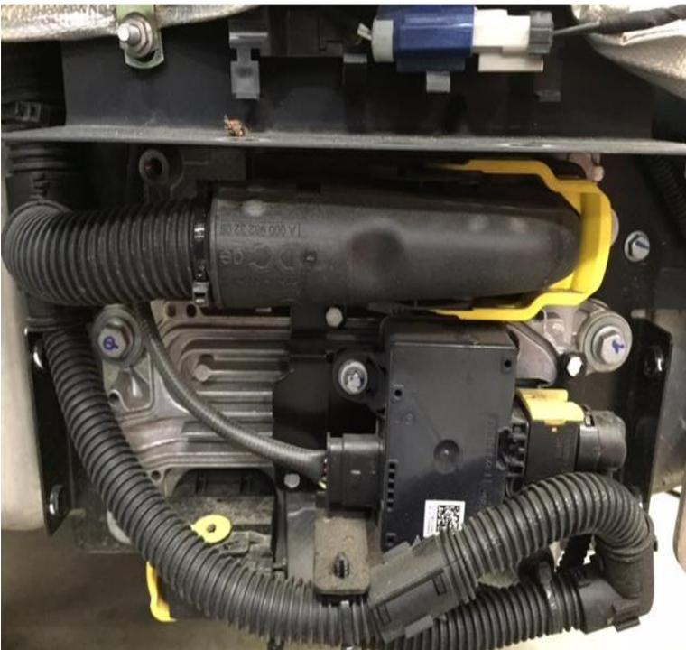
**Figure 3 – Harness Routing and Zip Tie Location**
