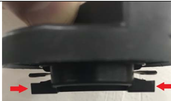
Improved Oil Fill Cap P/N A0000101485
