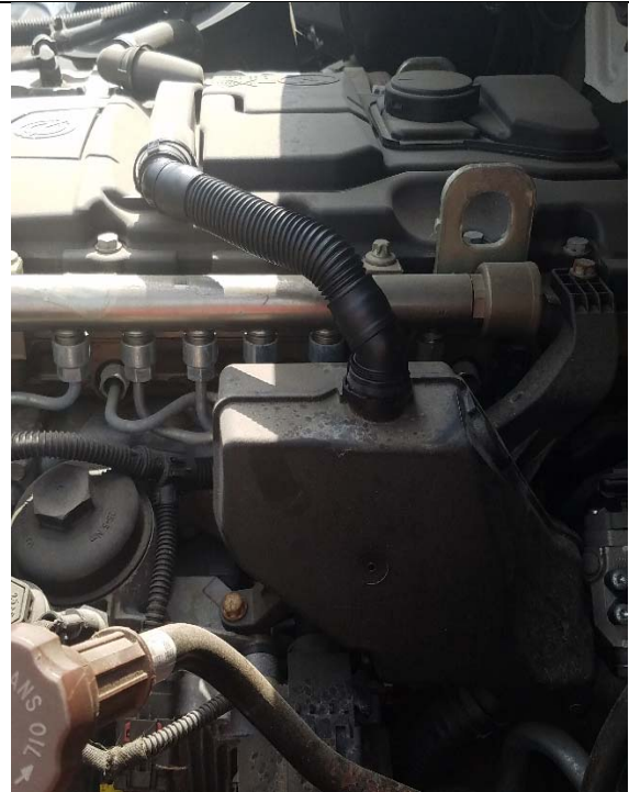
Improved Air Compressor Upper Suction Line P/N A9361306257
