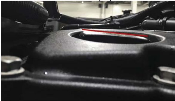
Figure 2 – Oil Fill Cap Correctly Latched
