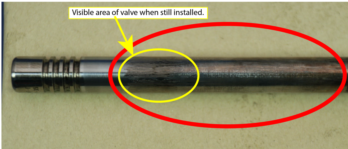
Figure 2 Valve Stem With Visible Wear
