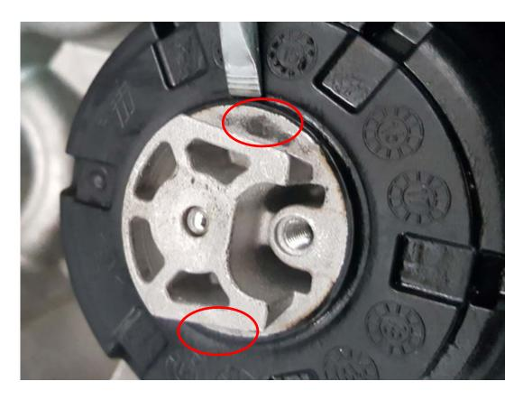
Put lubricating grease with graphite on red marked points as in pictures above.
