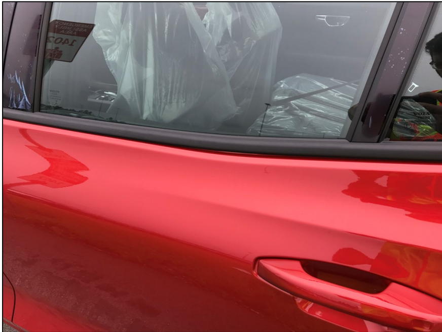
1. Identify car needing repair (loose OWS).
