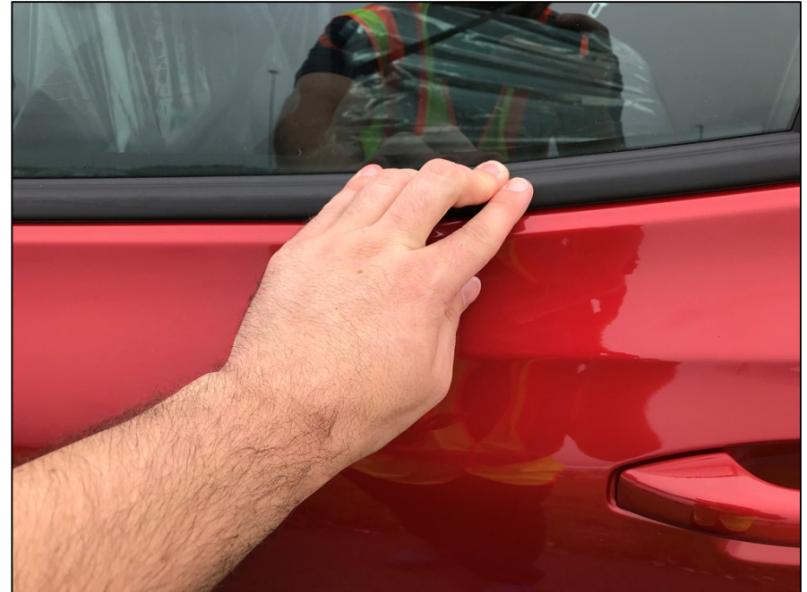
6. Reseat OWS. Use fingers to get to the initial position, and finish with a mallet.
