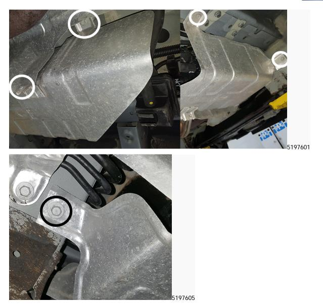
3. Remove the heat shield surrounding the Evaporative Emissions Canister by removing the five fasteners as shown.
