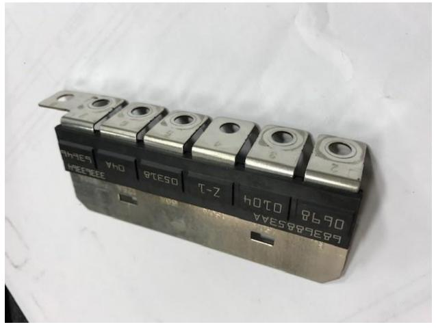
The fuse buss can be removed by removing all the nuts and sliding, removing the cables and then sliding it upward. Also note that the cable ends are indexed to only go in the correct location.
