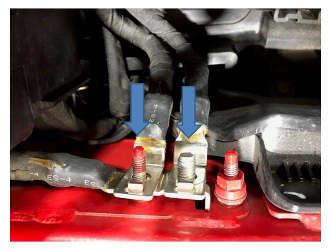
Be sure to isolate the wires from each other or the system will ground. One of these wires is a chassis ground.
