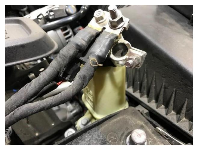
Then disconnect the 3 ground wires on the fender.
