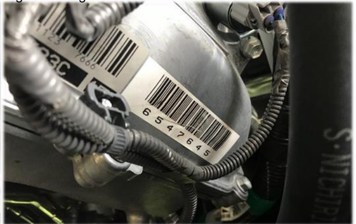
Figure 2: Engine serial number location – Zoom in
