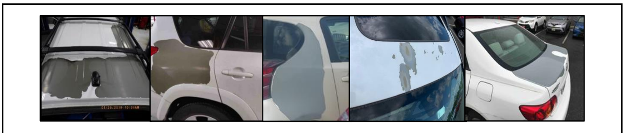
Figure 2. Examples of Affected Metal Body Panels Covered by This Service Bulletin
