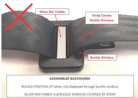
Figure 1 – Seat Restraint System Assembled Backwards / Incorrectly
