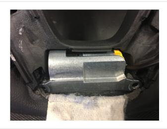
11. Image shows the vibration actuator with the insulation removed.
