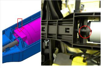
When seating the side with the electrical connector, slide the connector under a small tab as seen at left.
