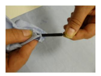
Lubricate the flexible drive shaft over its entire length using a lint-free cloth and P/N 83 23 9 407 810 Grease (NBU 12K)
