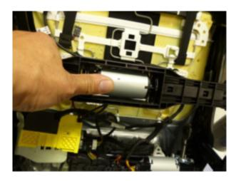
Remove the seat motor by pressing up from beneath.
