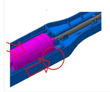
Press the motor down into the plastic housing (the bottom is open so you can manipulate it into place from top and bottom), sliding the side opposite from the electrical connector in first. The motor will click into place.
