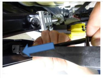
Insert the flexible drive shaft on an angle into the seat track assembly.
