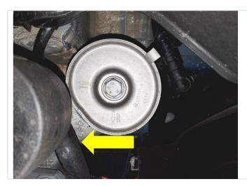
Was any visible damage to the anti-roll bar (arrow) noticed, paint / coating damaged?
