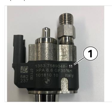
Do not replace any injectors that are index 11 and higher (1).
