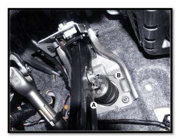
Loosen the fixed nuts (A) on the booster assembly. (Completely removing the nuts is not required).
