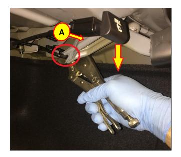
**6.** After releasing the hinge (A) from the torsion bar, slowly lift the torsion bar held by the vice grip and release the vice grip.
